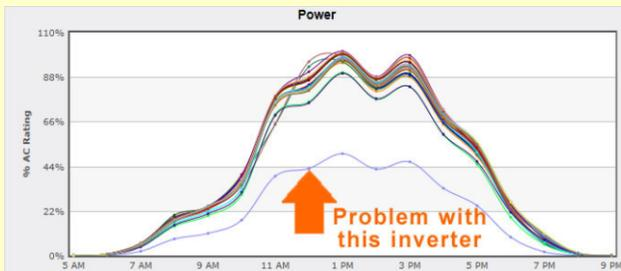
PowerWatch compares all inverter outputs to identify a faulty inverter. 30 day energy ratio log tracks intermittent operation.
